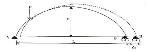
**Theory:-** The two hinged arch is a statically indeterminate structure of the first degree. The horizontal thrust is the redundant reaction and is obtained y the use of strain energy methods. Two hinged arch is made determinate by treating it as a simply supported curved beam and horizontal thrust as a redundant reaction. The arch spreads out under external load. Horizontal thrust is the redundant reaction is obtained by the use of strain energy method.
